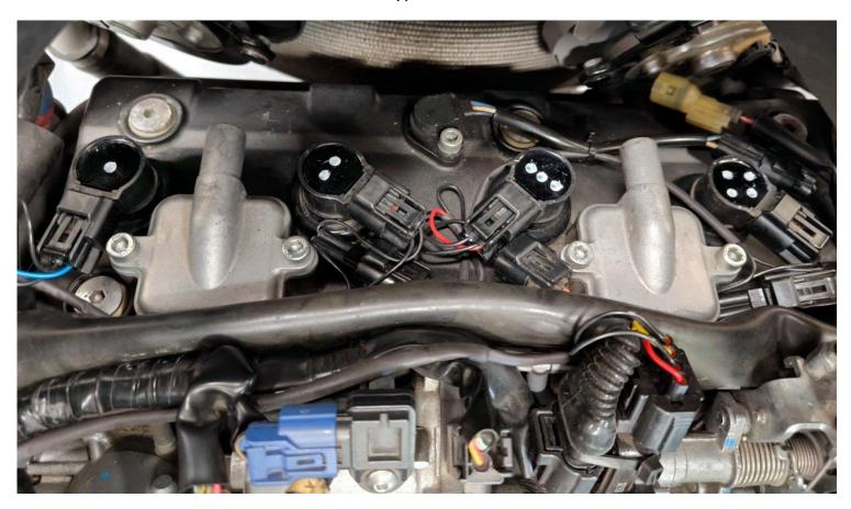
IMPORTANT NOTE: Make sure when plugging the connectors that you press them well enough to lock, this will provide sealed and reliable electrical connection, important for the function of the system. Find appropriate place for the control box and route the cables, they are high quality, automotive class cables however you must: Avoid moving parts as they might damage them, the best way is to follow other cables from the bike's harnes, use cable ties to fasten them. Make sure
